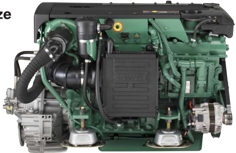
D4-300 with HS63AE reverse gear
